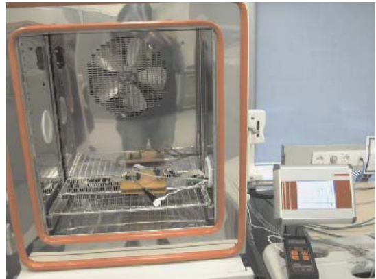
Set-up for temperature sensor measurements and characterization, including climatic chamber, logic analyzer, and other RFID test equipment.
